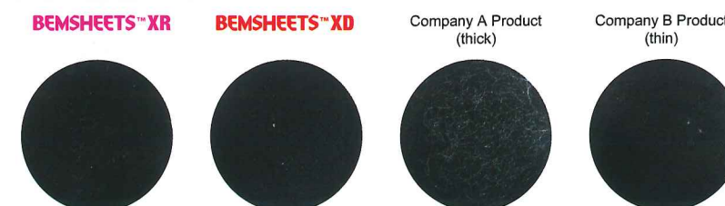
All of the samples were adjusted to 2cm x 4cm. They were then put in a flask filled of 200mL of deionized water and vibrated for 10 minutes in an ultrasonic cleaner under the conditions of 28kHz. Once the samples were removed, the solution was filtered through a black filter (φ3cm). The remaining fibers in the flask were also suction filtered after rinsing the flask twice with deionized water. After the filters were dry, the amount of remaining fibers on the filters was confirmed. (Own research)
